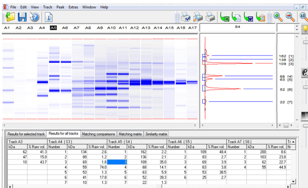
Figure 2: Lab901-GeneTools screen-grab of SD3 fractions 1 to 17. Protein analysis results are automatically presented by the ScreenTape P200 platform, without the need for a manual gel documentation system. All electrophoresis results are presented as a gel image. When a lane is selected it is displayed as an electropherogram (lane 5 has been selected in this view) where protein peaks are annotated with molecular weight (shown here) or quantity. All results are also displayed in a table containing data such as peak number, molecular weight, quantity and % purity.
